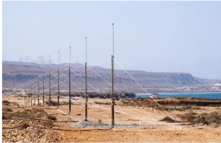
Figure 2.6— Typical land based radar wave measuring system [185]
