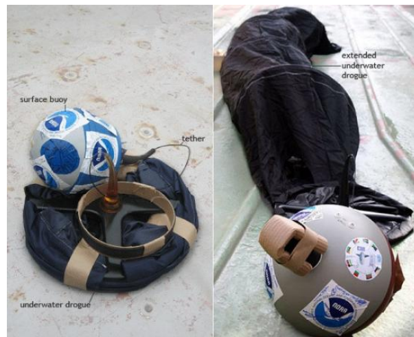
Figure 2.1 – A drifter neatly compressed for deployment ( left ) and with the nylon drogue fully extended ( right ), as it will be in the water once the cardboard wraps dissolve. [85]
