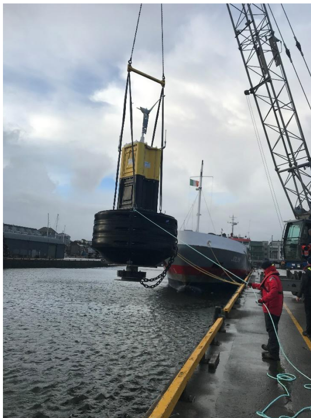
Figure. 3.52 The prototype WASP prior to testing at a benign site (Galway Marina)
