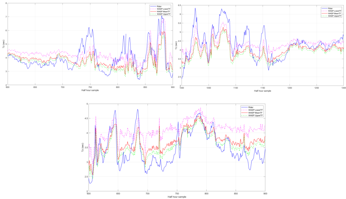
Figure 4.18 – Comparison between Waverider Tz and WASP mean, upper and lower standard deviation transfer functions generated Tz values for a single week, using selected March data energy rich in the frequency range 0.3-0.6 Hz applied to all WASP data for the months of April, May and June.
