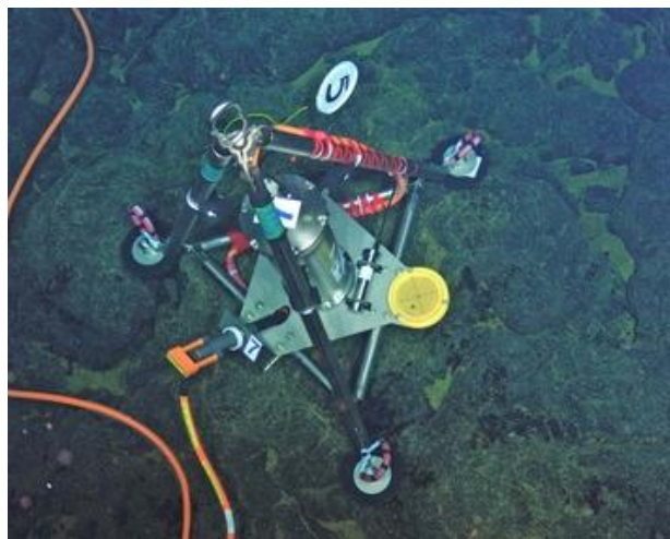
Figure 2.8– Typical seabed pressure sensor device [238]
