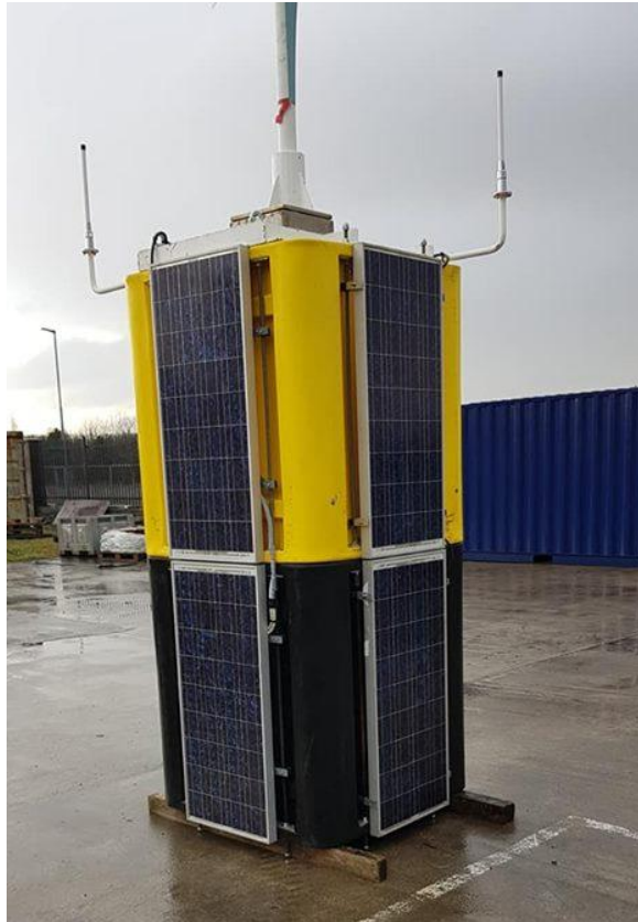
Figure. 3.53. Solar panels installed on the daymarks following removal of the wind turbine
