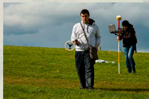
Above: Magnetic susceptibility survey in the vicinity of the trench. (Asia Balcerzak) Right: Magnetic susceptibility; contoured and coloured georeferenced map of part of the area showing zones of enhancement
