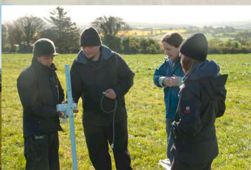
Above: Magnetic gradiometry; "am I non-magnetic?" (Asia Balcerzak) Right: Magnetic gradiometry; configuring a single gradiometer with 1m sensor spacing. (Michal Pisz)
