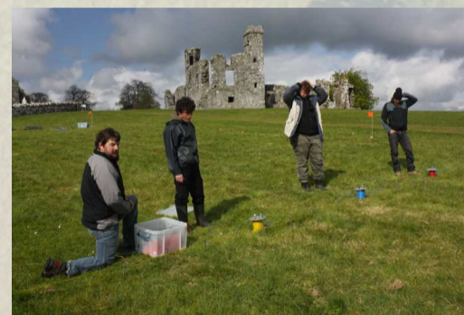
Above: Electrical Resistivity Tomography; "which electrode do we move next?" (Jaroslava Panisova). Right: South to north modelled pseudosection.
