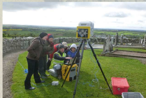
Terrestrial laser scanning; setting up a time of flight scanner at St Patrick's medieval church. (Anthony Corns)
