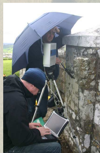
Terrestrial laser scanning; scanning the carved stone head in the graveyard wall with a triangulation mode scanner (Conor Brady)
