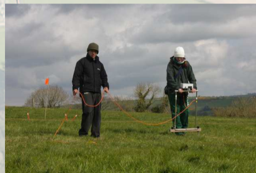
Above: Earth resistance; 0.5m twin-probe array survey over the trench. (Jaroslava Panisova). Right: Earth resistance image of part of the survey area showing a weak response from the trench and a strong response from a previously unknown parallel feature lying to the south
