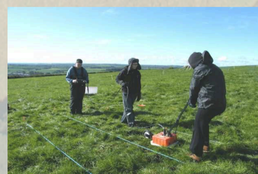
Above: Ground penetrating radar; control/data logger console, control/data cable and transmitting/receiving antenna mounted on a sled. (Séamus Ó Murchú). Right: GPR horizontal time slice showing the trench and numerous cross-cutting linear features.
