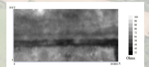
Above: Earth resistance; 0.5m twin-probe array survey over the trench. (Jaroslava Panisova). Right: Earth resistance image of part of the survey area showing a weak response from the trench and a strong response from a previously unknown parallel feature lying to the south
