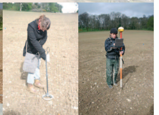
Above: Magnetic susceptibility survey (left), recorded using a dGPS and Toughbook laptop (right). (Conor Brady)
