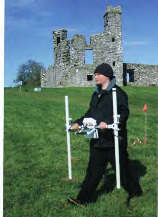
Below: Fig. 7—Earth resistance survey under way (Jaroslava Panisova).
