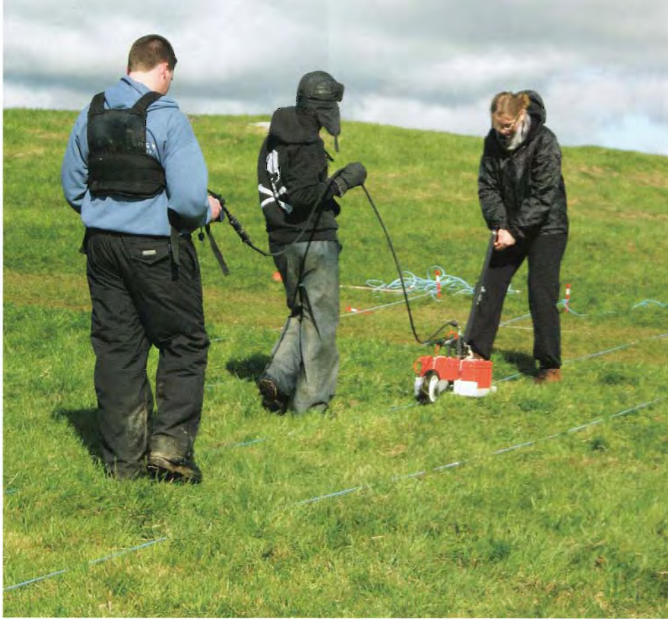
Left: Fig. 8—The ground-penetrating radar survey, with control/data-logger console, control/data cable and transmitting/receiving antenna mounted on a sled.
