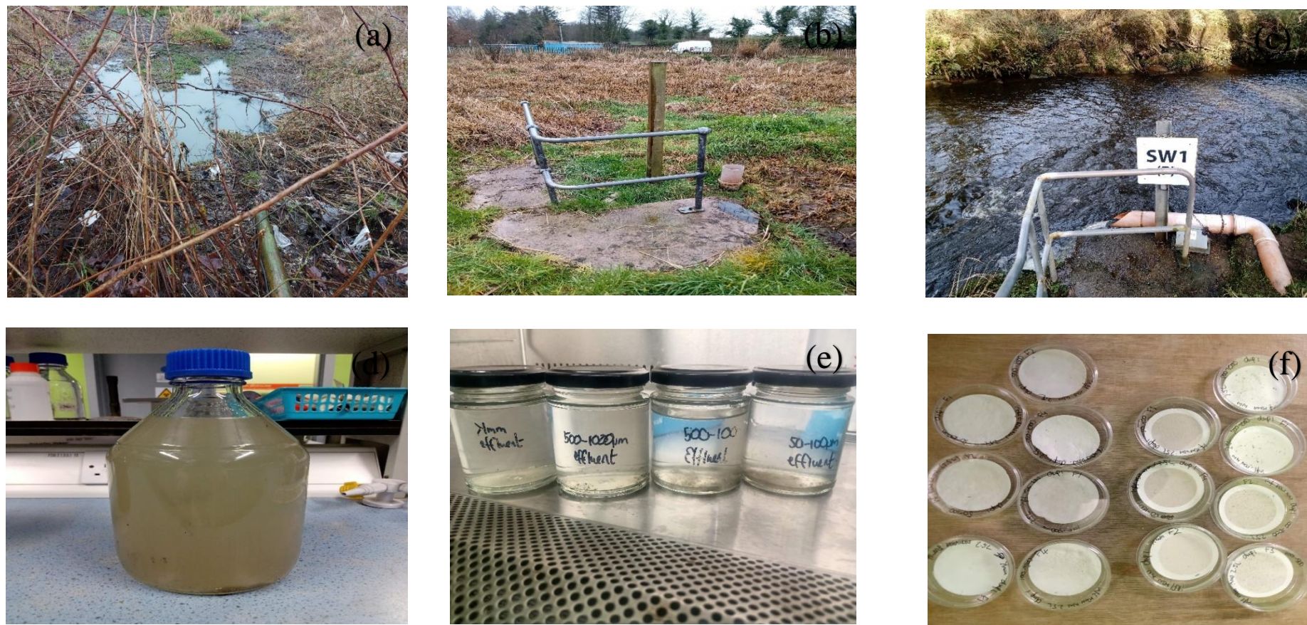
Appendix 9: Figure 1. From top left (a) raw wastewater influent sampling location with visible wipes and sanitary products, (b) sludge pond effluent sampling location, (c) treated water effluent sampling location, (d) raw wastewater influent sample, (d) residual particles from washed-down sieves used for treated water sampling, (e) sample filter papers containing microplastics pre- and post-digestion.
