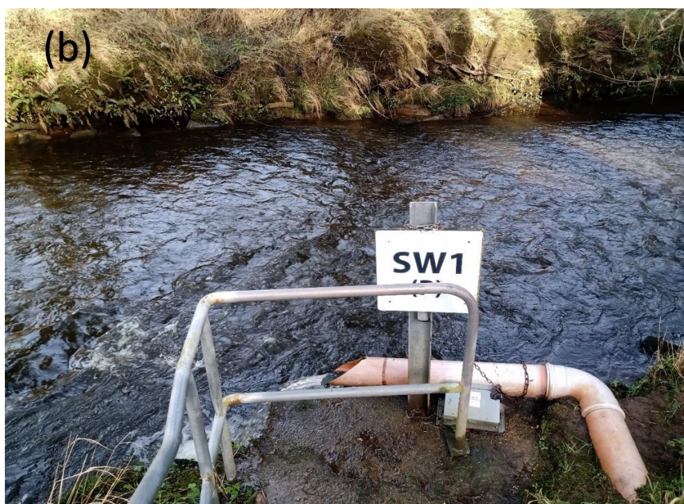
Figure 6.4: Two photographs of sample collection points: (a) the raw wastewater influent (b) the treated water effluent.
