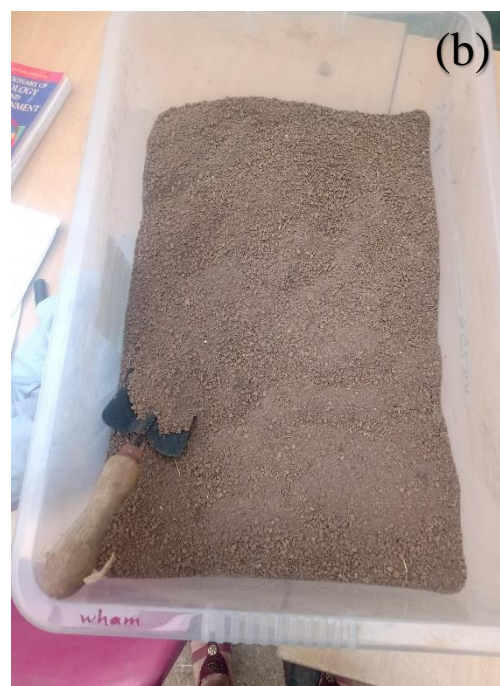
Appendix 7: Figure 2: (a) PE microfibres added to bulk soil sample pre-mixing (b) PE microfibres in bulk soil sample post-mixing
