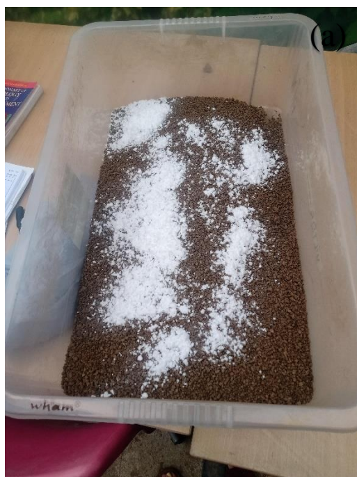
Appendix 7: Figure 2: (a) PE microfibres added to bulk soil sample pre-mixing (b) PE microfibres in bulk soil sample post-mixing
